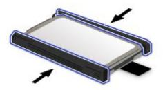
8. Insert the hard disk drive or solid state drive into the slot.
